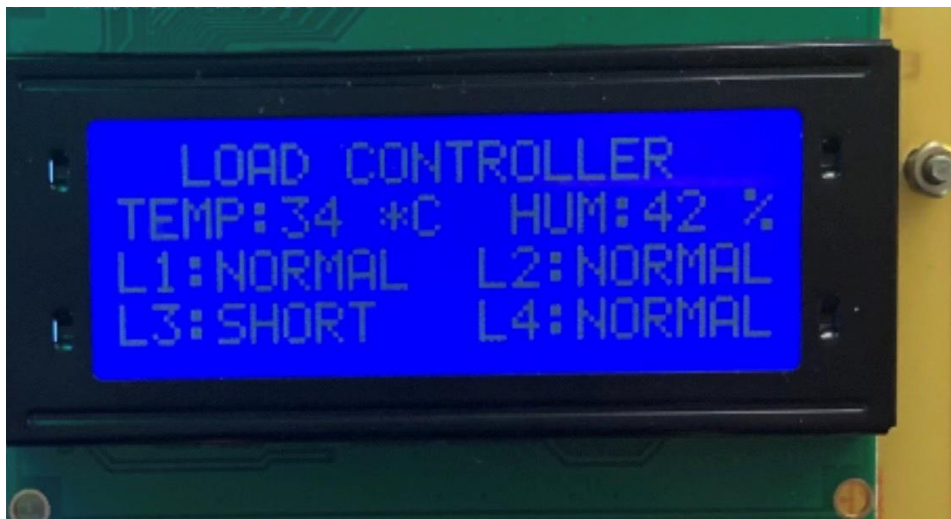
Figure 4.2 when circuit has short circuit
